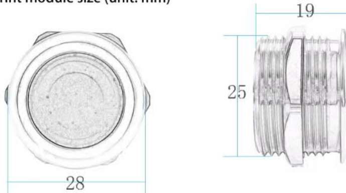
S4 Fingerprint module size (unit: mm)
