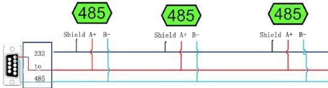
The COM port of a computer is generally RS232, so you need a 232-485 converter for connection (an active and isolated converter is recommended for industrial environments). After conversion, RS485 has A and B two wires, A is connected to the board A terminal, and B is connected to the board B terminal, the 485 shield can be connected to GND. If there are more equipment, it is recommended to use shielded twisted-pair cable and a chain network structure.
