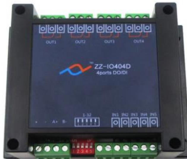
The module adopts the standard Modbus RTU protocol, the communication interface supports RS485 or RS232, and supports communication baud rates of 2400, 4800, 9600, 19200, 38400 (default 9600). Each relay output is independent and can be connected to different load devices, such as 220V electric lights, 24V solenoid valves, etc. Both AC and DC devices can be controlled. Each relay output contact is isolated, and can set 0-255 device addresses. It also supports flash on/off function.
