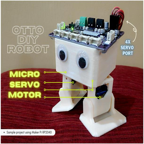
The board is compatible with the existing Pico ecosystem, Software, firmware, libraries and resources that are developed for Pico should work seamlessly with Cytron Maker Pi RP2040 too. CircuitPython is preloaded on the Maker Pi RP2040, so it's very easy to get started. The board supports commonly programming languages as well, so you are free to use MicroPython and C/C++ for Pico/RP2040.
