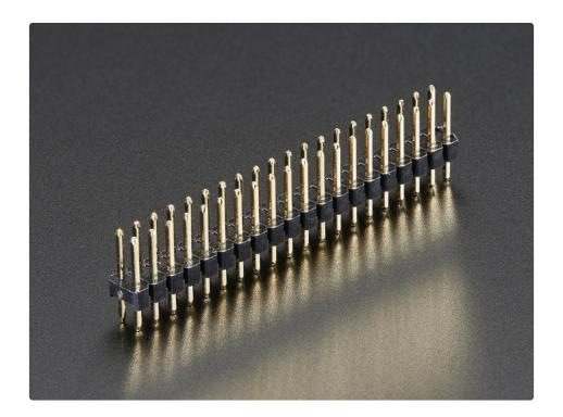
Once soldered in, you can plug in any HAT or topper. The pinout is completely identical to the 2x20 headers on the Pi 2 and Pi A+ & B+
