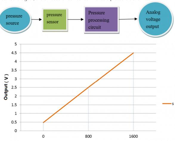
Input (Atmosphere Pressure + Tested Pressure) (kPa)
