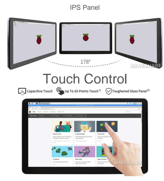
1) up to 10-points touch, depending on the operating system. 2) up to 6H hardness toughened glass panel.
