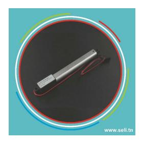
This time DFRobot brings you an electric push rod. Despite a mini body, it comes with a thrust of up to 128N and a stroke of 100mm when powered by a voltage of 6V.
