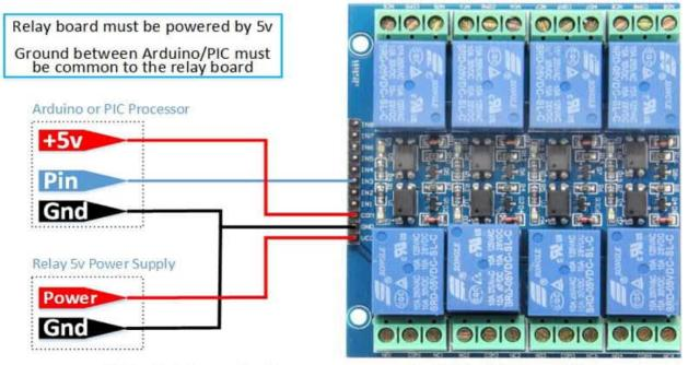
Relay is triggered when processor pulls IN1 to IN8 line LOW
