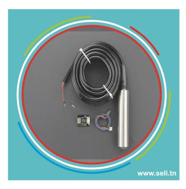
This throw-in type liquid level transmitter adopts high-performance pressure sensing chip, with advanced circuit processing and temperature compensation technology. The level transmitter receives different pressures at different depths of liquid, which can be converted into corresponding current signals and output through the sensor. In this way, the depth of liquid can be measured.
