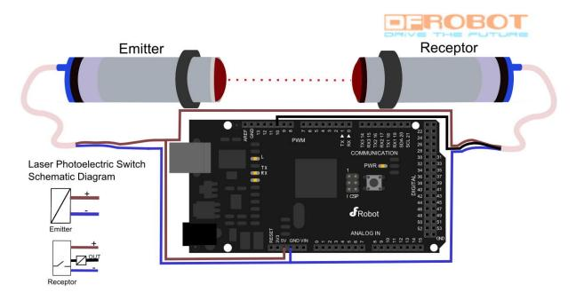
The output pin of the laser photoelectric switch is connected to pin 10 of the Arduino board. The LED on 13 pin will reflect the state of the output pin. Try to block the laser and watch the effect. The Receptor will output high level when it detects laser signal.
